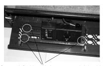
Secure left side with 2 screws and right side with one screw.
